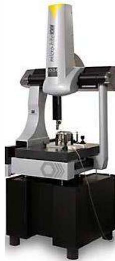
Our new Brown and Sharpe MicroHite DCC CMM has a measuring volume of 17"x19" by 15.5" high, with PC-DMIS software. It is a great complement to our Mitutoyo BHN-710 CMM which has a volume of 27"x39" by 17.7"high, and was recently upgraded with MCOSMOS software, which is also PC-DMIS compatible. Both CMM's have custom reporting, so customers can review electronic or hardcopy printout report of measurement data for their parts.
